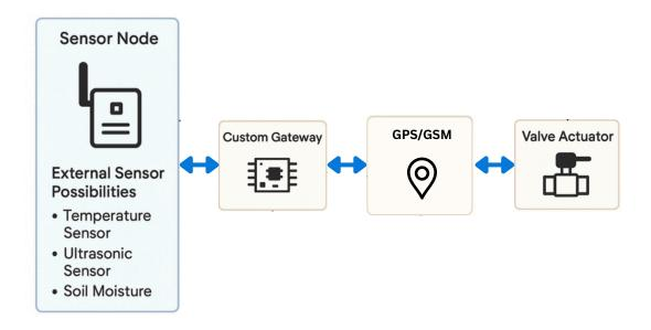
It communicates wirelessly over roughly 15km line of sight using a custom LoRa P2P protocol to a custom gateway. This enables off-grid, real-time automation such as smart irrigation, and while it doesn't require internet, it can connect if desired.
